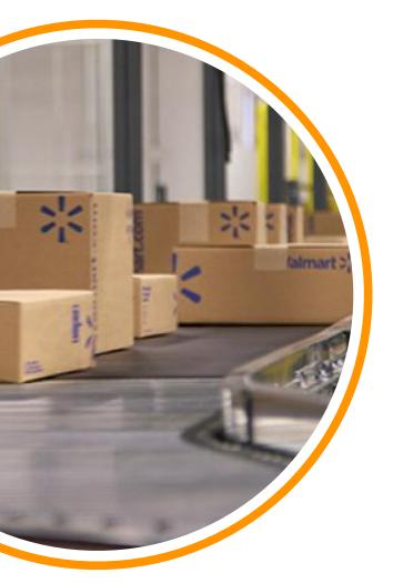
With a conveyor speed of more than 2 m/s, the IMPEL's belt curve is designed for high performance and trouble-free operation in different applications. The curves are available in several widths, angles and weight classes.
