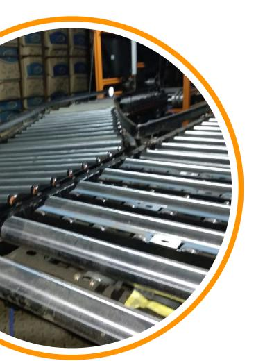
The merge is used for connecting lateral roller tracks at an angle (30° or 45°) to the main track. This can be used for moving material off the track (e.g. with HPD (High Performance Divert)) or onto the track.
