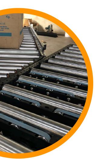
The intelligent 24V Roller Conveyor family (straights, curves and merges) offers highest **energy efficiency** for unit-load handling (boxes, totes, crates, etc.). Its exemplary low-noise operation and maximum safety due to low voltage make this technology a key element for an improved working environment for your operators. Note that all IMPEL's roller conveyor modules are also available as non-driven conveyors, where unit loads are moved by gravity or manually.
