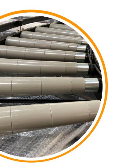
The 24 V roller conveyor curves change the direction of transport of the material. The conical rollers retain the alignment of the materials between side frames. A controller enables zero pressure accumulation transport. Each zone is powered by a 24 V RollerDrive that is connected to a fixed number of idlers via round belts.
